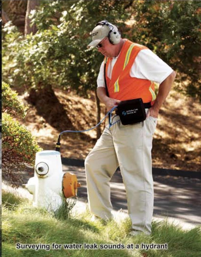
Surveying for water leak sounds at a hydrant
