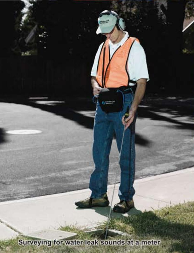
Surveying for water leak sounds at a meter
